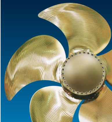
**5 bladed CPP**. Wärtsilä offers a wide range of 5-bladed propeller hubs. Through this design the power is spread over 5 blades instead of over 4 blades, whereby reducing vibrations in aft ship and accommodations. It also reduces underwater-radiated noise levels. For vessels with stringent noise requirements, a fully flush contour of the 5 bladed hub is available.
